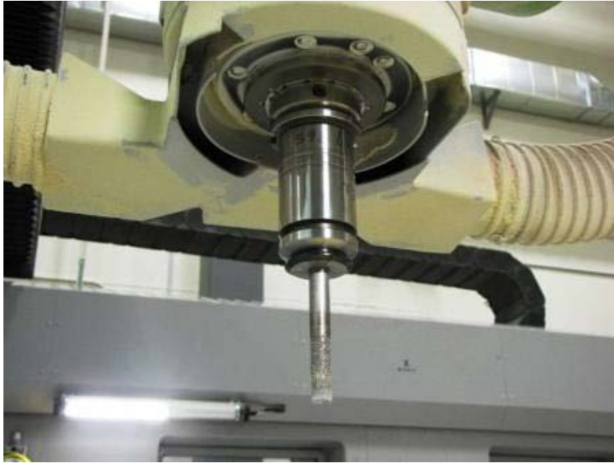
Figure 6 Cubic boron nitride bit in FZ32 core mill
