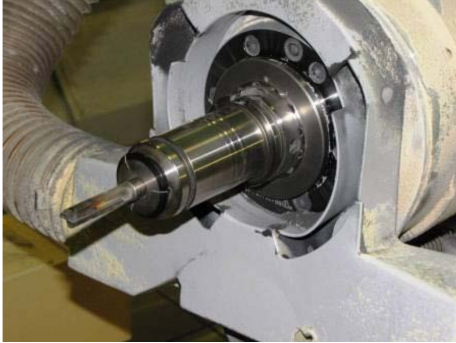
Figure 8 Polycrystalline diamond bit used for majority of ACM panel cutting
