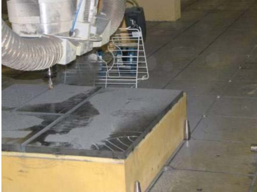
Figure 9 FZ32 cutting graphite-epoxy panel, showing cloud of particulates
