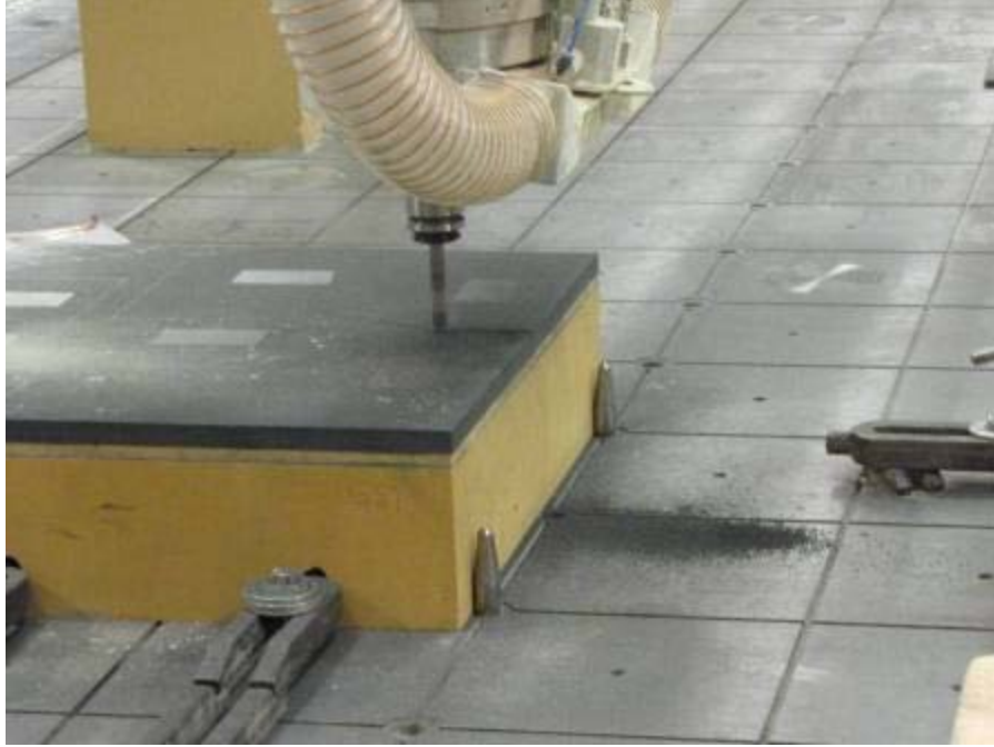
Figure 7 Cutting ACM panel with CBN bit
