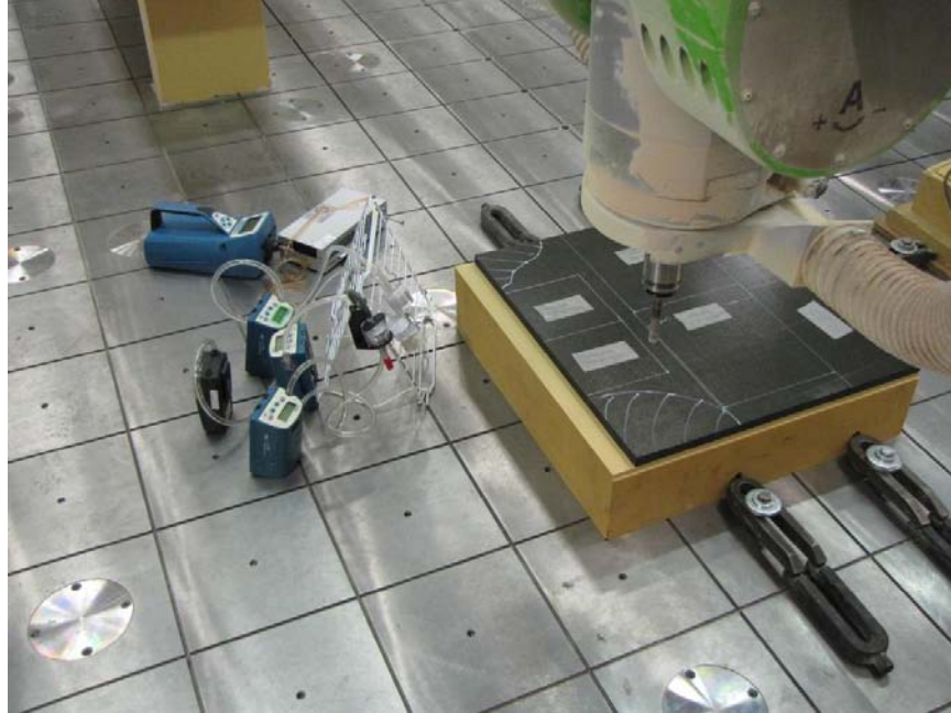
Figure 4 Initial setup of the aerosol sampling apparatus
