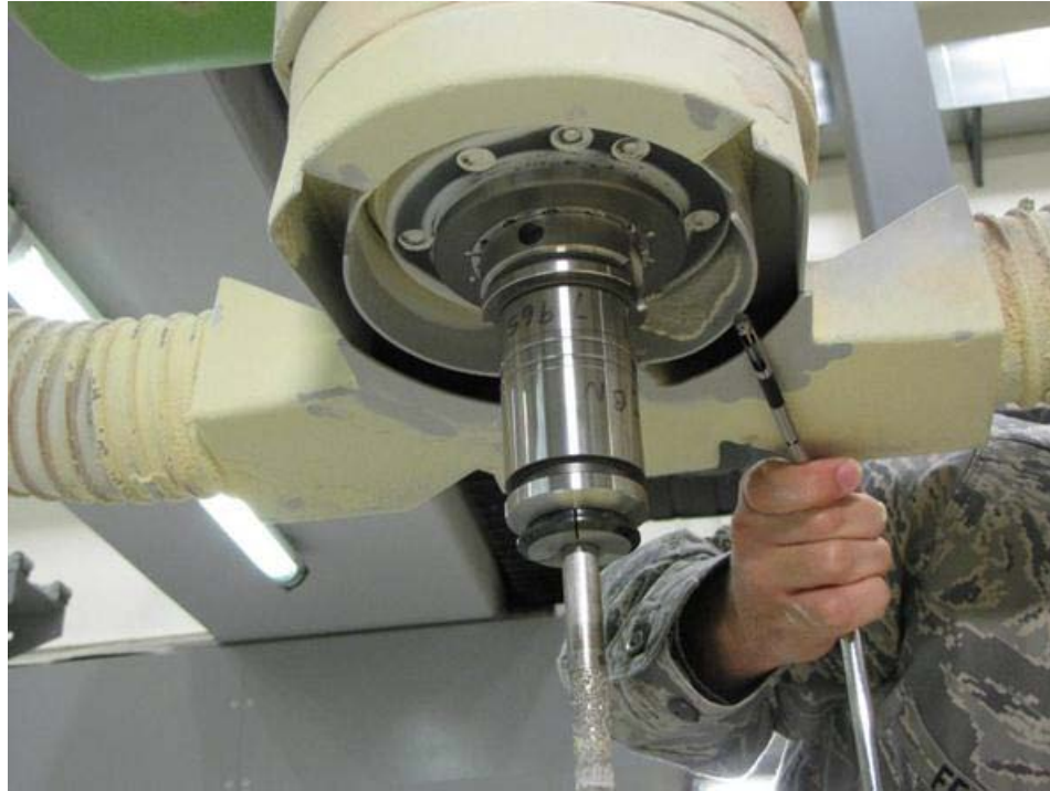
Figure 2 Measuring face velocity of FZ32's LEV
